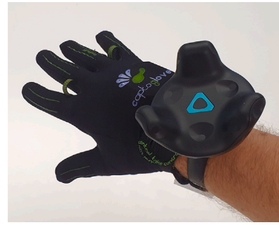
Fig. 8. Sensors used for the implementation of the system: CaptoGlove and HTC VIVE Tracker 2.0.
