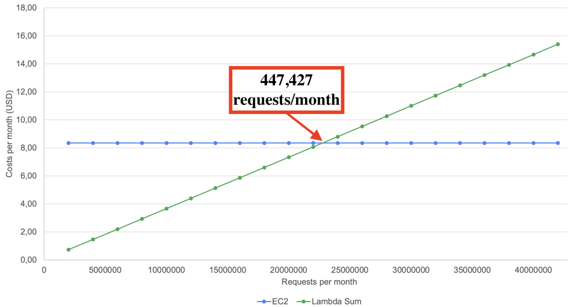
Figure 4.3. Costs Comparison of AWS EC2 and Lambda. The intersection is the point where the expenses of running the Lambda services are as great as running the EC2 service for one month, and beyond it that it becomes more expensive. The cost of the EC2 remains static regardless of the amount of internet traffic that it receives.
