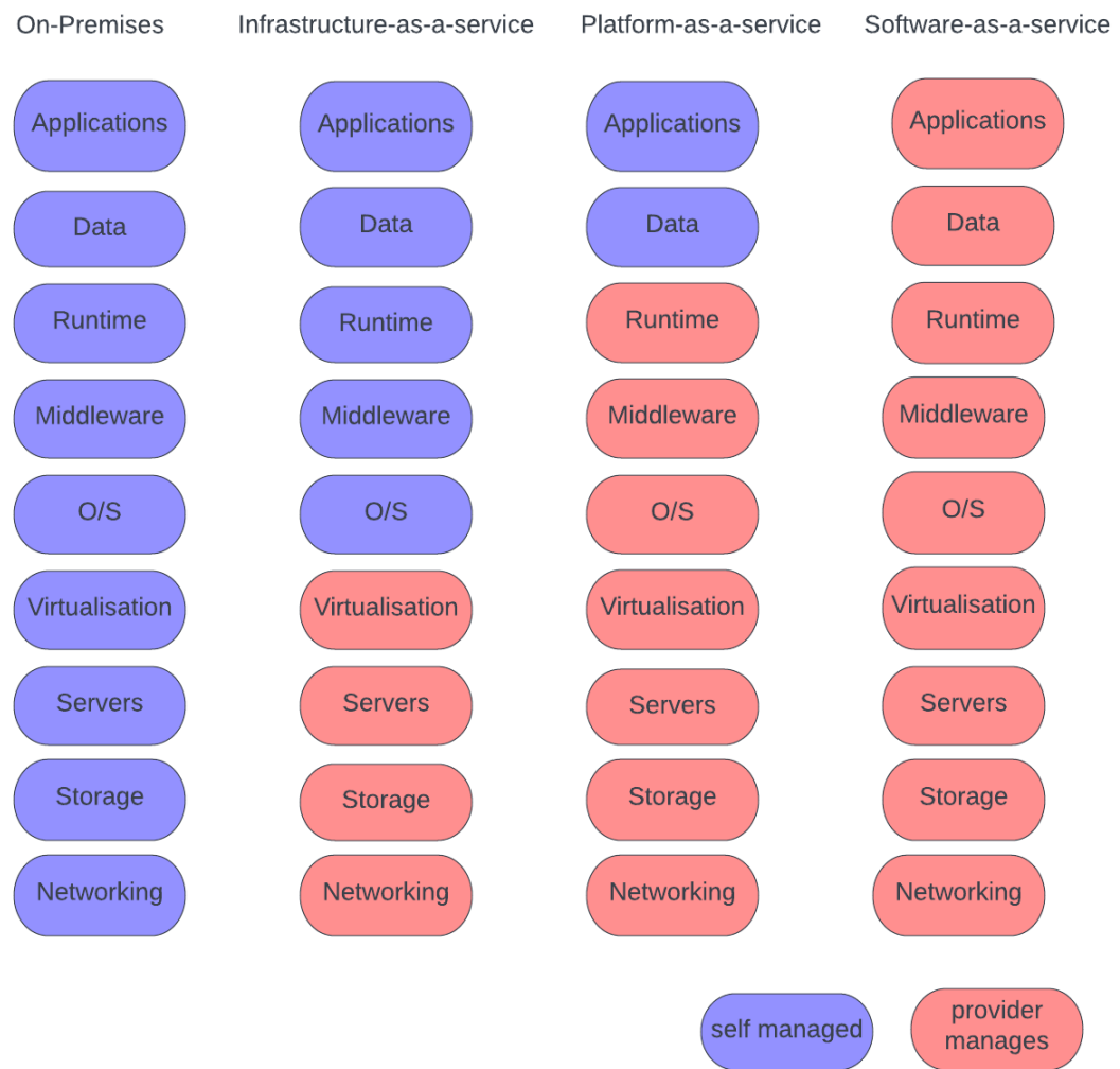
Figure 1.1. A representation of different types of cloud services and what components of the hardware and operating system are under the control of the end-user and which components are entirely controlled by the service provider.
