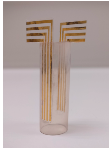
Figure 8. Trial 1 electrodes attached on the inner wall of a FEP tube to enable simultaneous OPT and mFEIT imaging.
