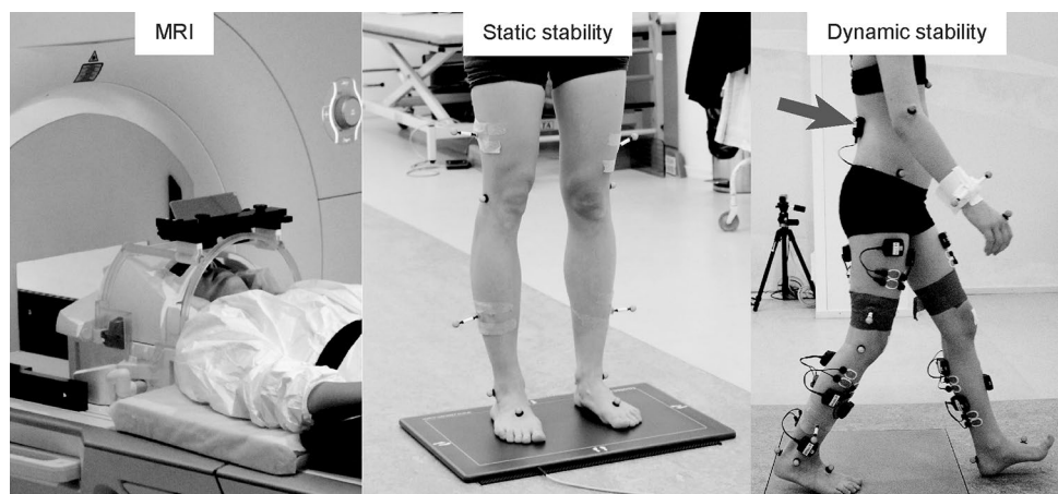
Fig. 1 Experimental setups in MRI, static stability and dynamic stability measurements. The arrow indicates the location of inertial measurement unit on the lower back of the subject during dynamic gait stability testing
