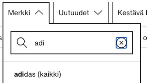
Figure 4. Accessibility error zalando-E2: In the search bar of the brand ("Merkki") filter the "X" button does not do anything. However, this is a general bug because the button does not work for mouse users either. Users can erase the text with backspace.
