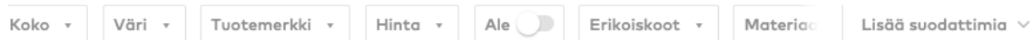
Figure 38. Accessibility error aboutyou-E4: By default, some of the filters are hidden and the show more filters button is placed after the hidden filters. The focus is lost in the hidden elements while the user navigates to the button.
