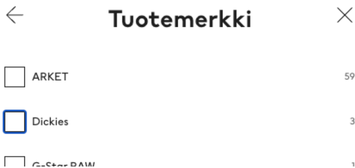
Figure 13. Accessibility error hm-E2: Each list item with a checkbox has two focus areas instead of one which causes unnecessary clicks for a keyboard user.
