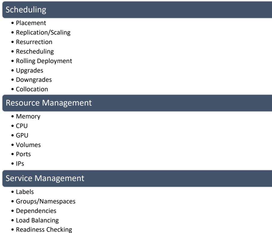
Figure 15. Orchestration tool can handle scheduling, resource management and service management tasks (Isenbeg, 2017).
