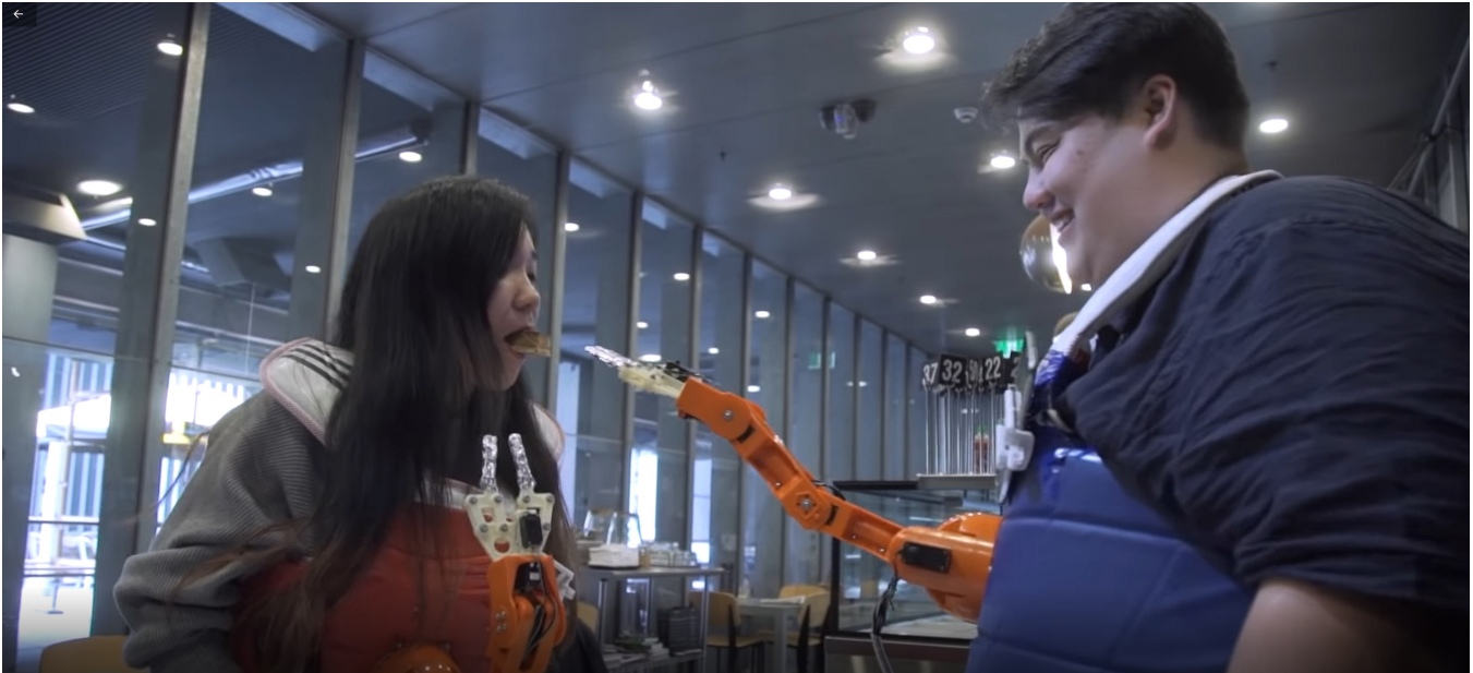
Figure 2: Two players are eating food by using the robotic arm of Arm-A-Dine
