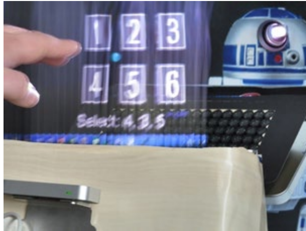
Figure 6. From front left to back right: Leap Motion controller, FogScreen, phased ultrasonic 16x8 array, and projector (masked with an R2D2 printout) (Sand et al., 2015a).
