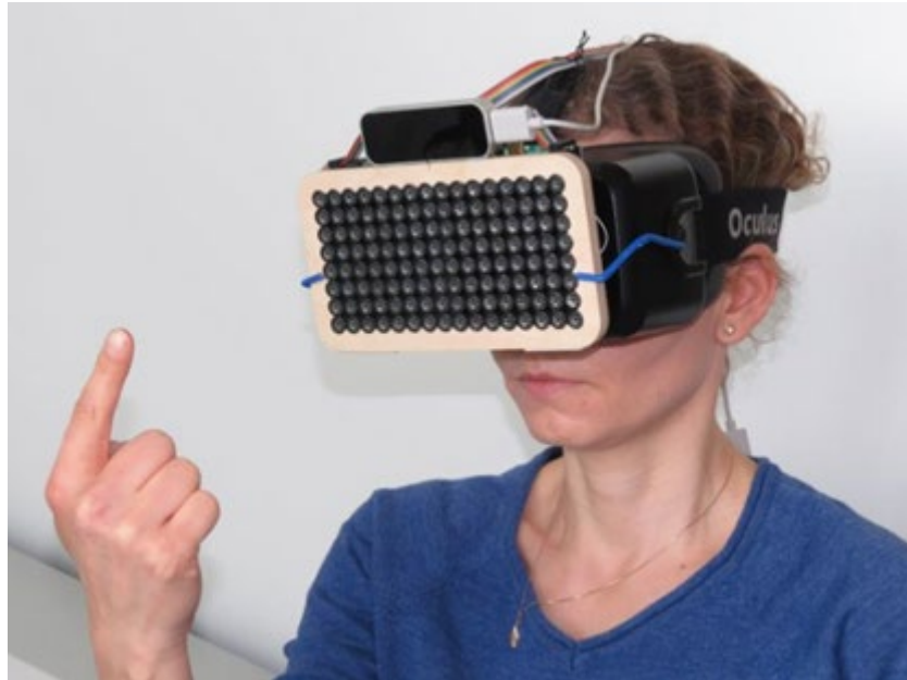
Figure 5. An ultrasonic mid-air haptics device attached to a head-mounted display always keeps the feedback oriented to the facing direction. The hand tracking sensor on top of the matrix allows the focal point to be directed at the fingertip.
