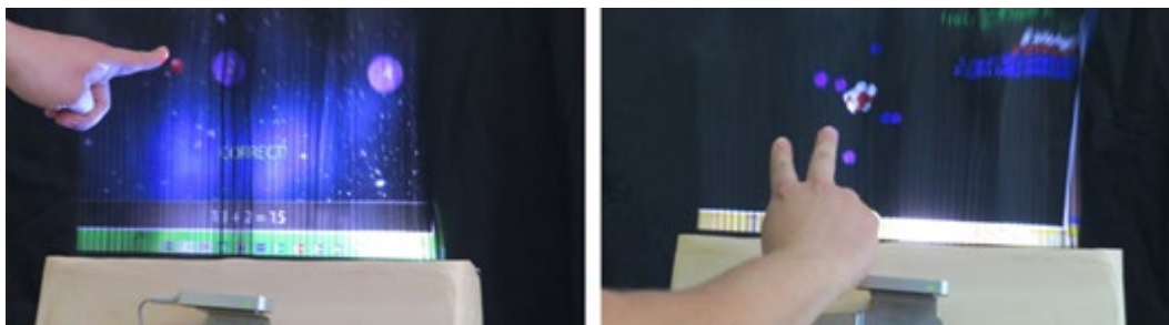
Figure 3. Left: an interactive math learning application on a 17" desktop FogScreen with hand tracking. Right: an atomic model visualizer with gestural interaction.
