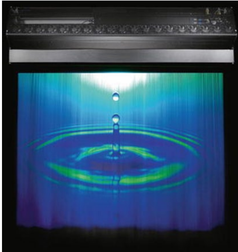
Figure 2. A large fogscreen hanging from the ceiling can show a clear projected image on a thin layer of fog.
