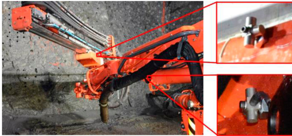
Figure 2. Underground rock drill (Sandvik) and 3-axial accelerometers (Ojala et al. 2017a). (Images are available in colour online)
