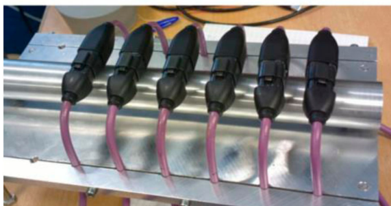
Figure 5. Test samples in the test rig used in the multivariate static test. (Images are available in colour online)
