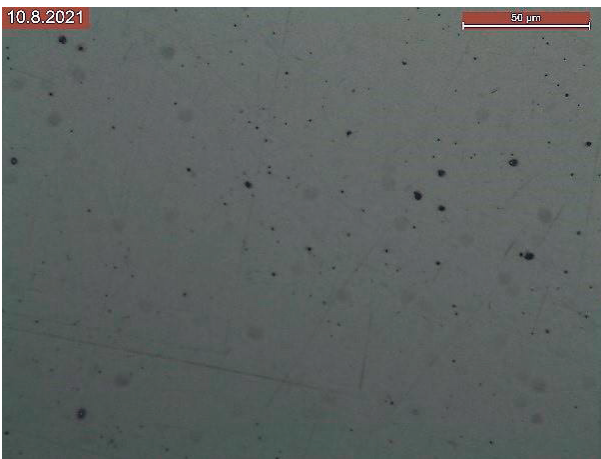
Figure 85. Optical image of RF-sputtered \text{Al}_2\text{O}_3 sample 040821A1 of 0.85 \mu\text{m} deposited at 125 \text{ }^\circ\text{C} .
