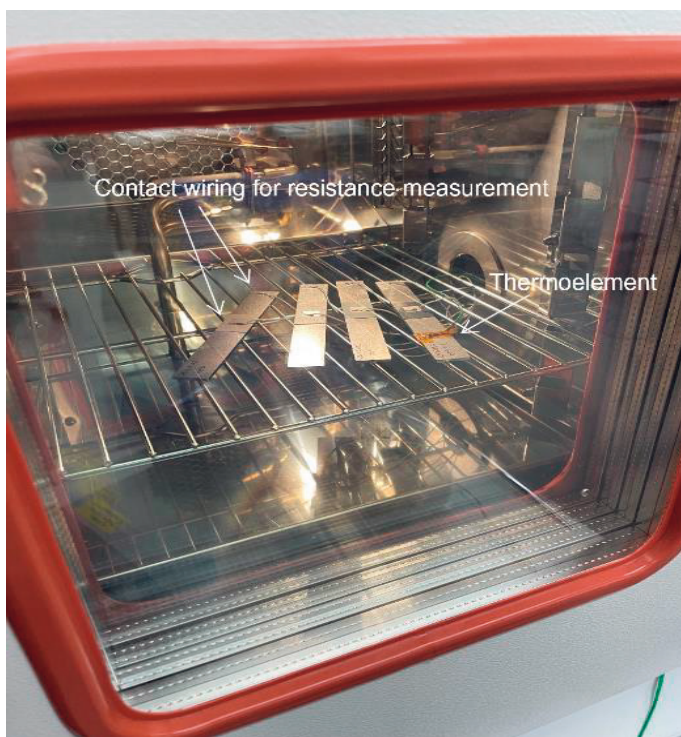
Figure 54. Placing of APS samples in resistance measurement with type K thermoelement in Vötsch VCL 4003 climatic test cabinet.
