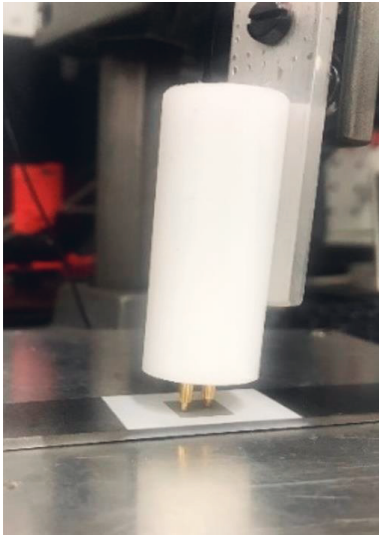
Figure 22. Two-point measurement of sheet resistance of Ti6Al4V contact electrode on HVOF- and APS-deposited aluminium oxide coatings.
