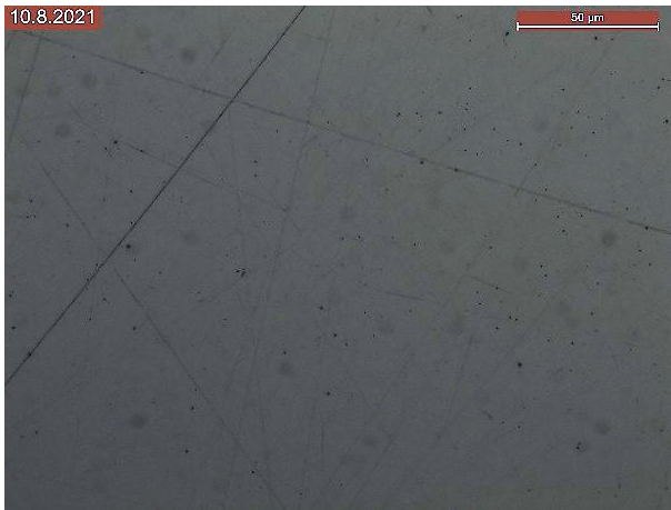
Figure 86. Optical image of RF-sputtered \text{Al}_2\text{O}_3 sample 050821A1 of 1.3 \mu\text{m} deposited at 250 \text{ }^\circ\text{C} .
