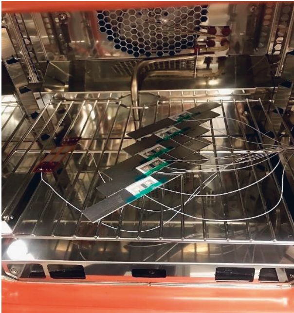
Figure 72. Resistance measurement of piezoresistive hard carbon thin film thermistors on HVOF and APS insulating coatings to determine thermistor beta value.
