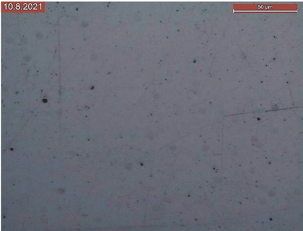
Figure 84. Optical image of RF-sputtered \text{Al}_2\text{O}_3 sample 120721A1 of 0.58 \mu\text{m} deposited at 20 \text{ }^\circ\text{C} (RT).
