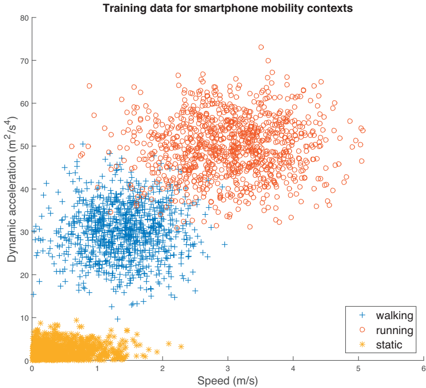
Fig. 3.1: Example training data for supervised learning. The data are similar to those shown in Table 3.1. Note the partial overlap between the “walking” and “running” classes.
