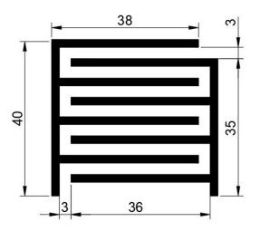
Figure 2. Interdigitated sensor geometry (dimensions in mm).
