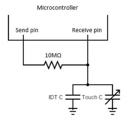
Figure 5. Measurement circuit of each individual sensor.
