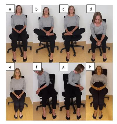
**Figure 6.** Measured sitting positions during the smart chair test. (**a**). Ergonomic posture, (**b**). Right leg crossed, (**c**). Left leg crossed, (**d**). Detach from the backrest, (**e**). Sit on the edge, (**f**). Lean to the right, (**g**), Lean to the left and (**h**). Lean back and sit on the edge.
