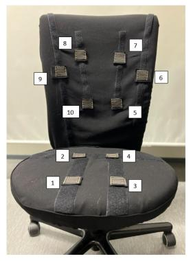
Figure 1. Smart chair with sensor distribution and number identification.
