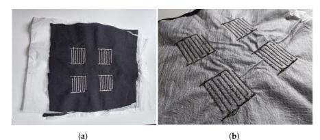
The support fabric could be removed afterwards by being diluted in water. The final presence textile capacitive sensor (PreCaTex), embroidered can be observed in Figure 3.
