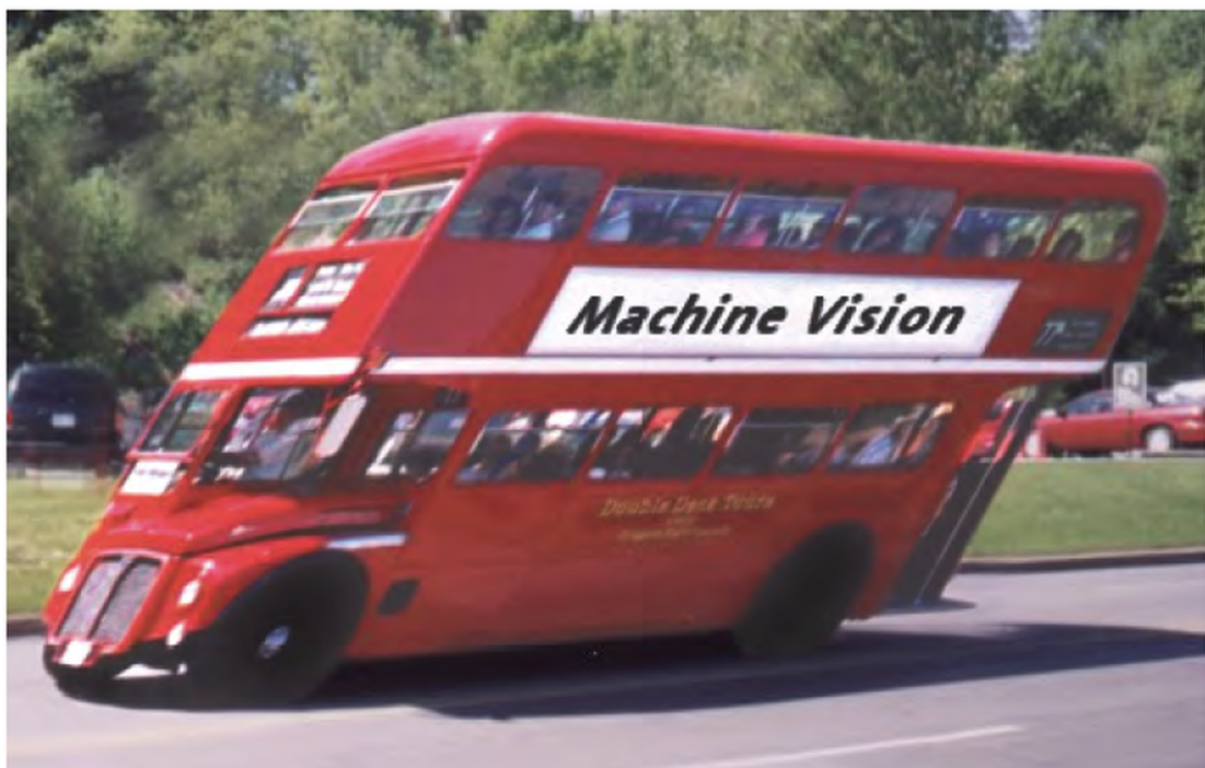
Figure 2.2. Image of a fast-moving object taken with a rolling shutter camera [11]
