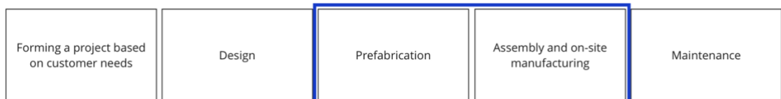
Figure 2.2 The phases of a construction project of a residential building with prefabricated concrete element frame modified from (Teriö et al., 2003).
