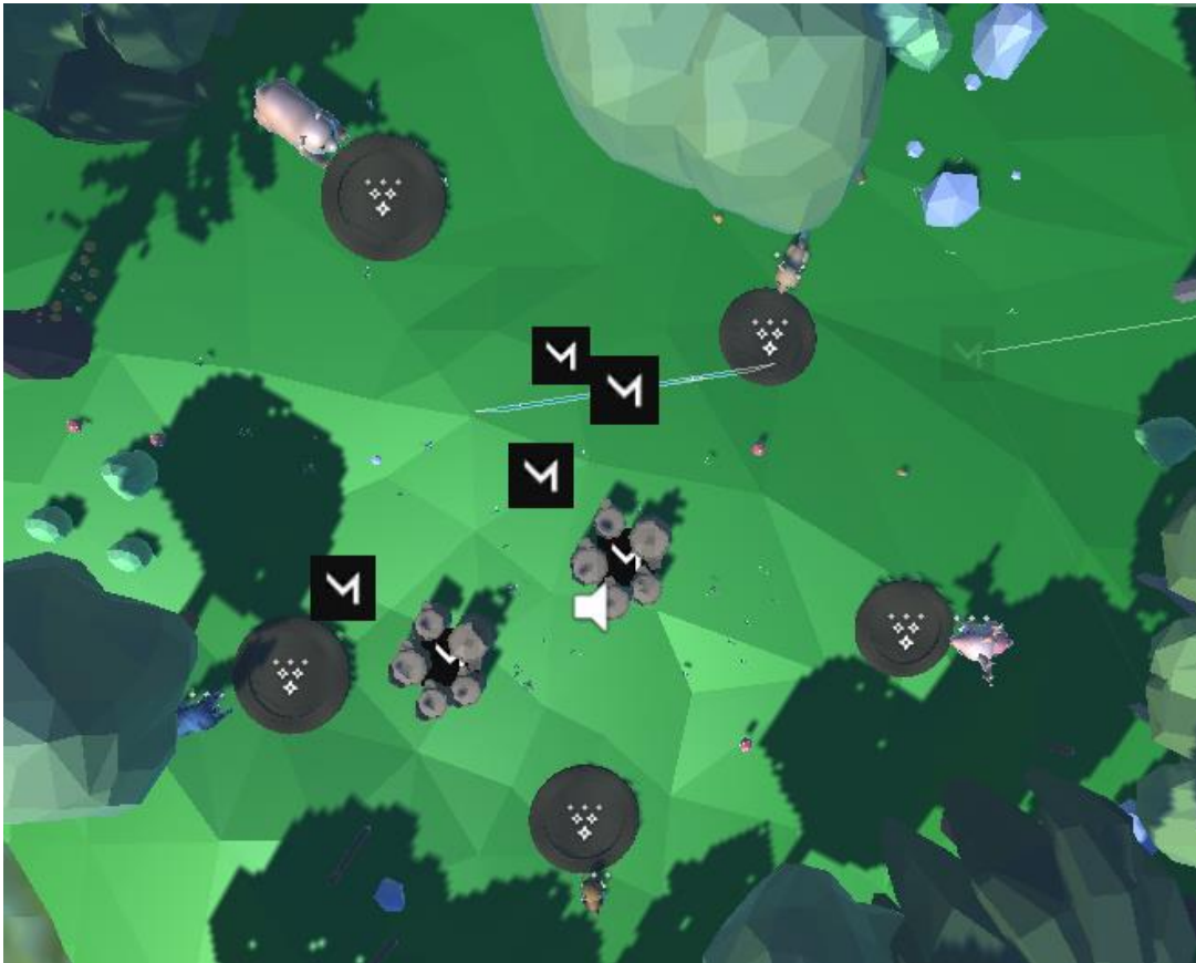
Figure 7: Multiplayer Scene from above in Unity editor. Black squares with letter M are GO's that use Mirror's Network Identity component and are not shown in the game.
