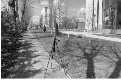
Fig. 2. Location at which the range of the devices was measured. The devices were placed at distances between 5–220 m along the pathway.
