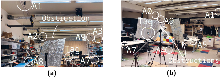
Figure 5.8 Setups used to acquire NLOS measurements. The setup in Figure 5.8a corresponds to position P1 from Figure 5.4. It includes one aluminum panel placed as a blocker between anchor A_1 and the tag. Figure 5.8a corresponds to the position P4 from Figure 5.4. It includes two aluminum panels that block the initiating anchor A_1 and various anchors depending on the tag’s position on the rail.
