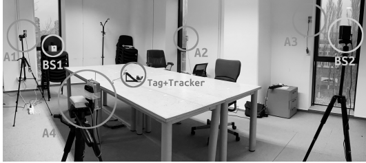
Fig. 8. Localization setup: the four anchors (A1 to A4) encompass an area of approximately 4.5 \times 3.6 m and the tracking area is on the table. The ground truth was acquired using two HTC Vive base stations (BS1 and BS2) and a tracker that was colocated with the UWB tag, shown on the table.
