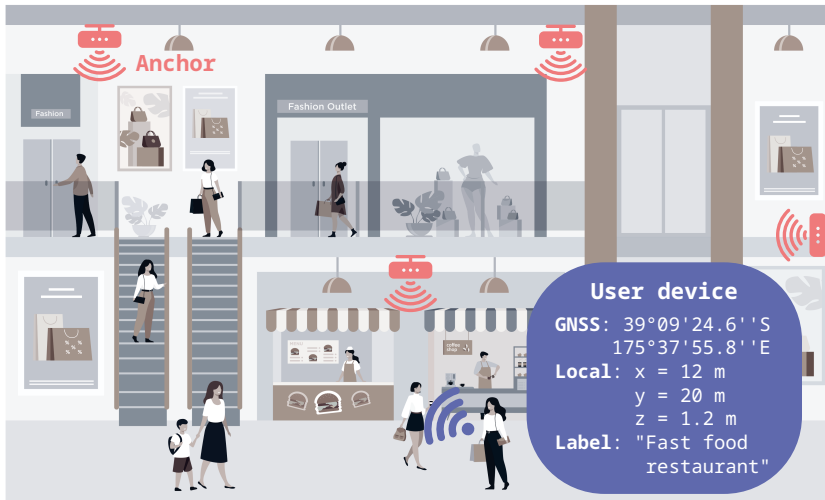
Figure 2.3 Practical localization scenario in everyday life. Several UWB anchors are deployed as part of the infrastructure. The user device (also called a tag) needs to be equipped with a UWB transceiver. The localization system provides the user either their position using global coordinates, local coordinates (relative to the building), or as a label depending on its proximity to surrounding landmarks.
