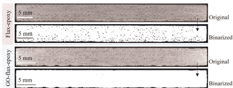
Fig. 3. Internal porosities of flax-epoxy and GO-flax-epoxy composites based on X-CT tomography.
