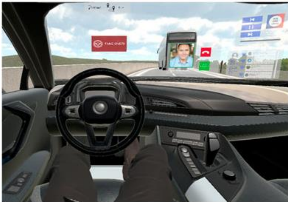
Figure 5. A concept of windshield display showing the capabilities of world fixed information and periphery information (Riegler et al., 2022)
