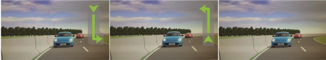
Figure 32. “Explicit communication” versions. Arrow pointing in a perceived direction (left), Arrow pointing to the actual driving direction (middle) and no augmentation at all (right) (Wintersberger et al., 2018)
