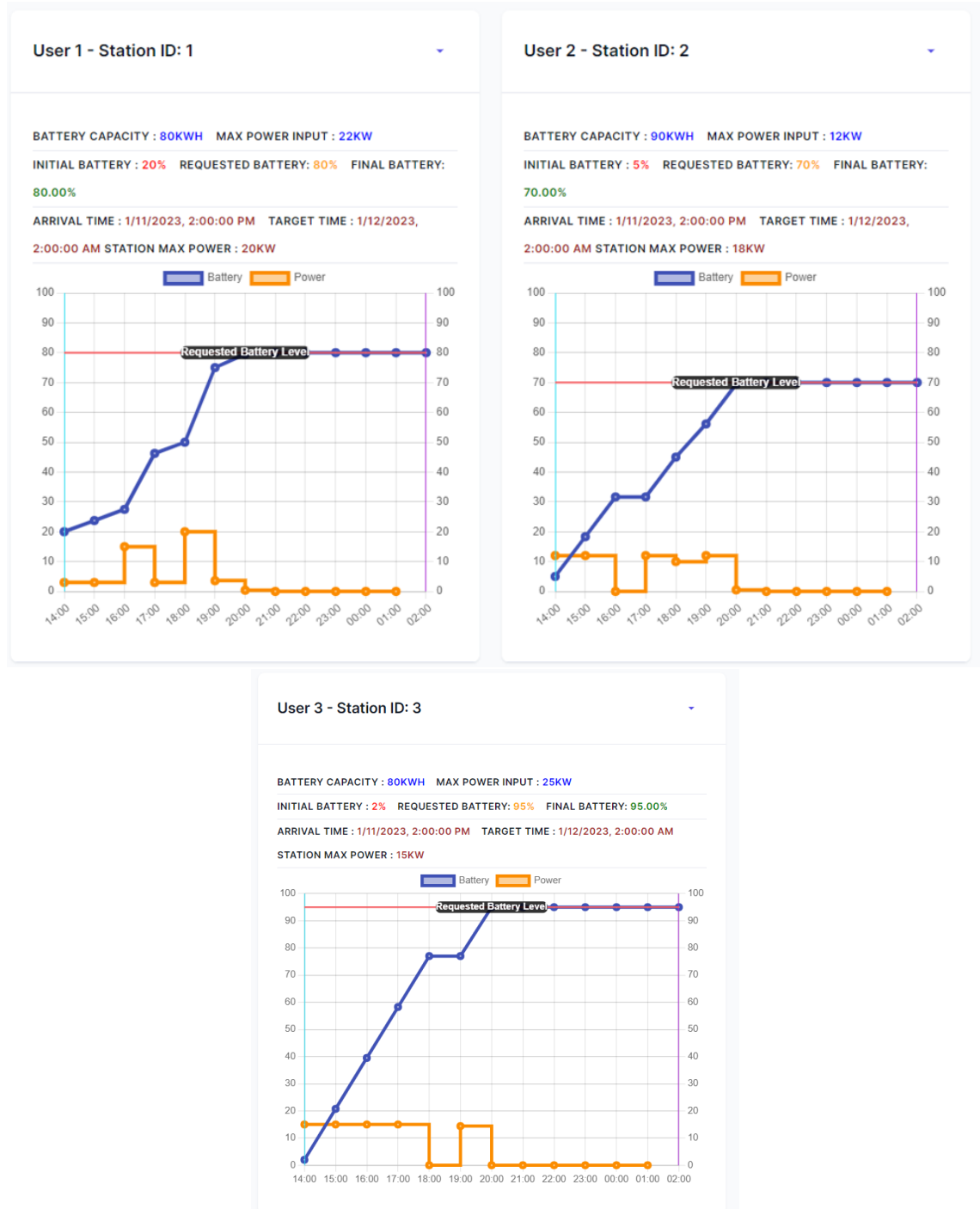
Figure 3.9. Power output and battery status for User 1, User 2, and User 3 in simulation scenario 1
