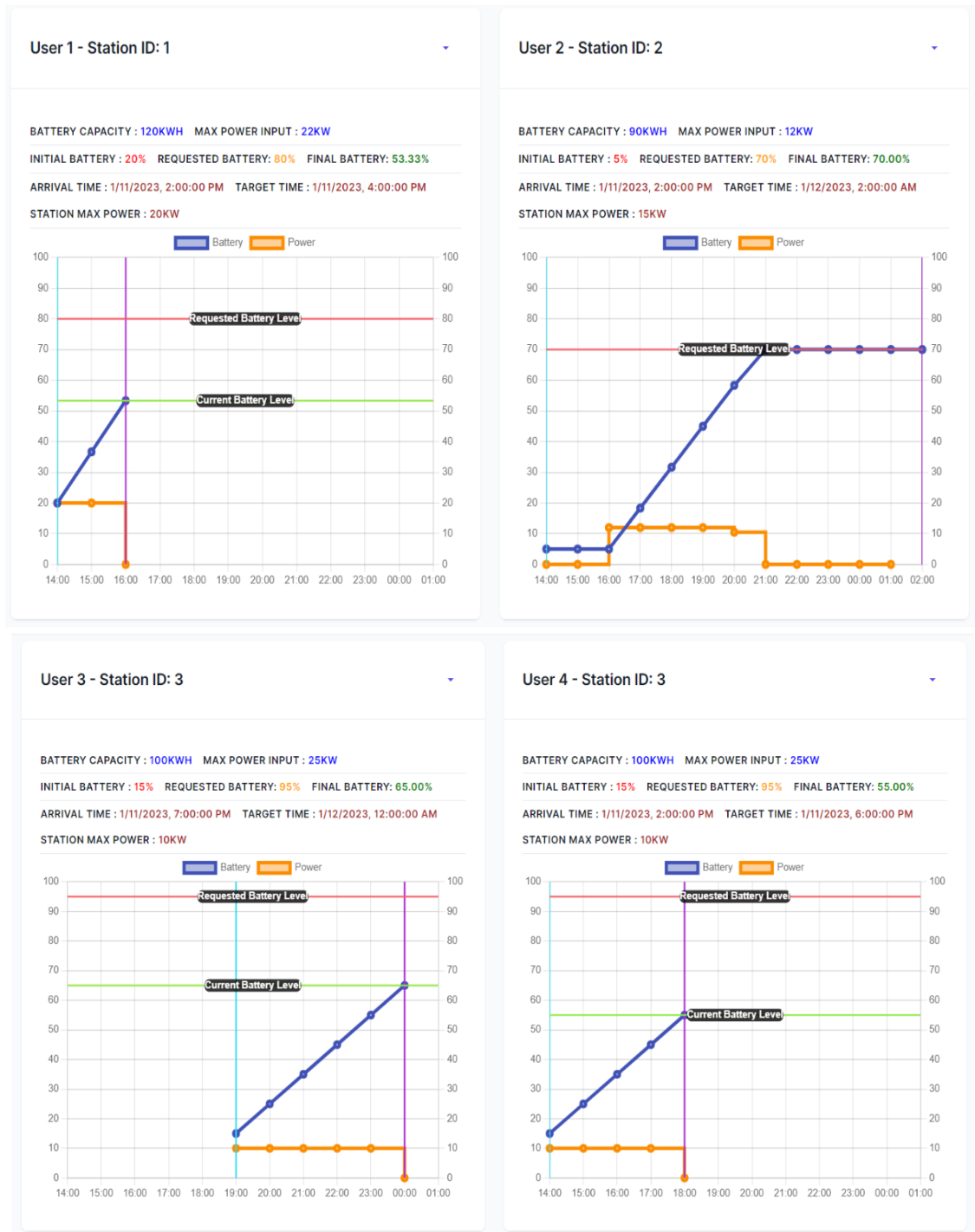
Figure 3.11. Power output and battery status for User 1, User 2, User 3 and User 4 in simulation scenario 3
