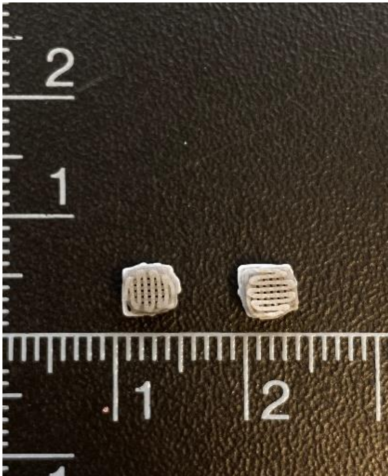
Figure 1. 1. Photograph of two gridded sintered logpile scaffolds (size: 5.7mm x5.7mm x5mm)
