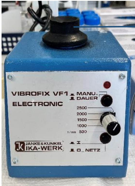
Figure 3. 1. Photograph of the Vibrofix VF1 mixer. The bottle (that has pluronic and the glass) is touched on the black part on the top when it is spinning with 2500 rpm
