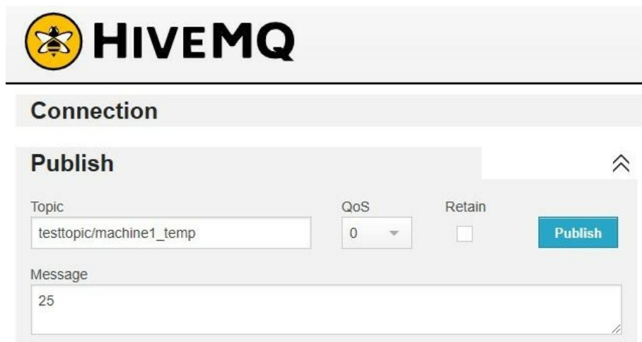
Figure 31. Testing with HiveMQ MQTT Broker
