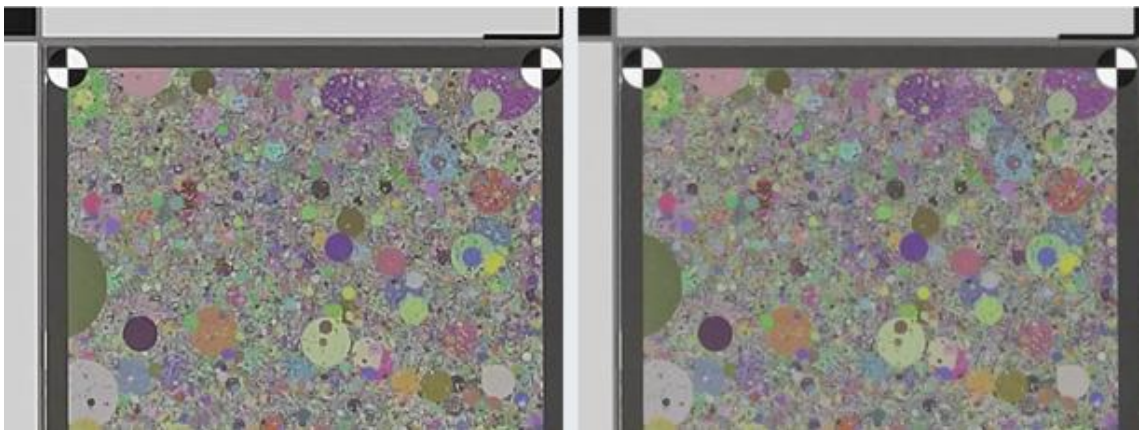
Figure 6.7. Comparison of the texture targets between tuning solution generated using only DISTS (004) on the left and tuning generated using only VCX score as the target metric (002) on the right. Images were taken under bright illumination. Note how higher sharpening on the left produces better textures.
