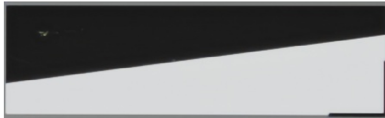
Figure A.2. High contrast slanted edge target cropped from TE42-LL test target.
