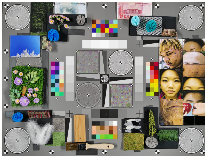
Figure 6.1. The verification test chart used to assess the final image quality.
