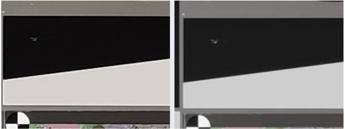
Figure 6.6. Left image is the commercial OnePlus 7T (001) baseline image, right image is generated with the tuning solution achieved using only VCX score as target metric (002). Images are taken under bright illumination. Note the differences in the edge shape.
