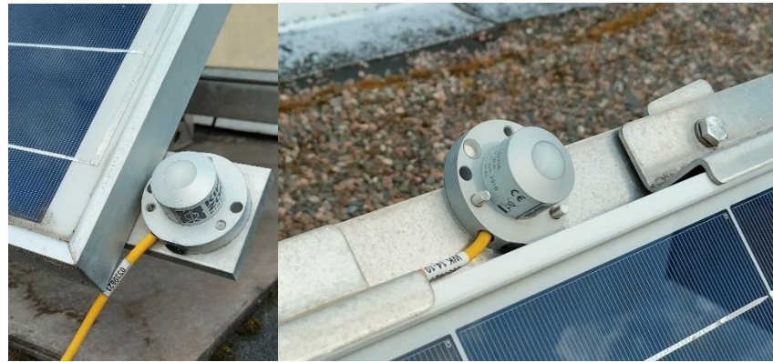
Figure 5.1.3. SP Lite 2 sensors mounted on side (left) and the top (right) of PV modules.
