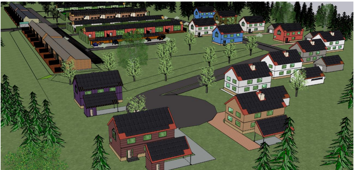
Figure 5.1. Aerial view of the simulated suburban area with PV modules on the rooftops facing south.
