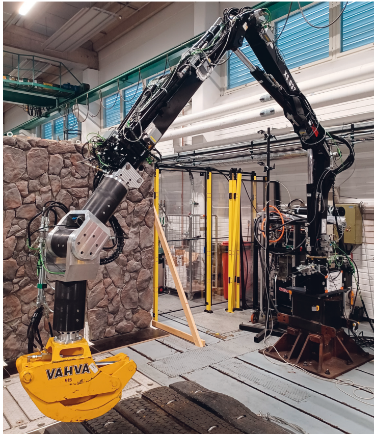
Figure 1.2 Hiab 033 XS manipulator in laboratory of Tampere University.
