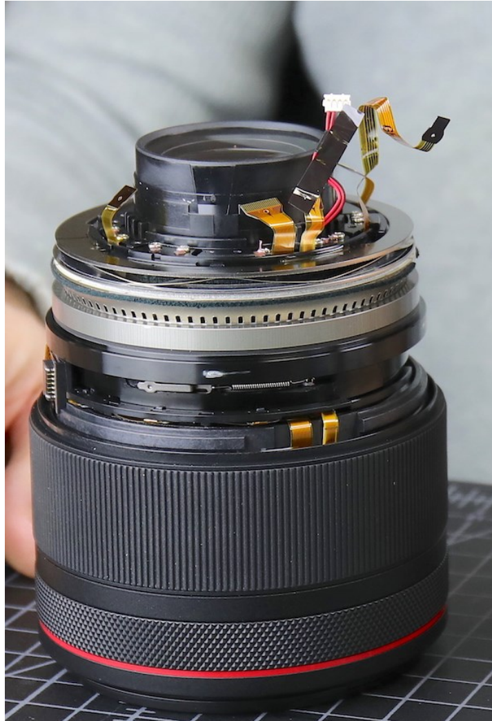
Figure 38. Side view of the Canon RF 50 mm 1.2L. From the partially disassembled lens you can see the toothed ring of the ultrasonic autofocus motor. [57]
