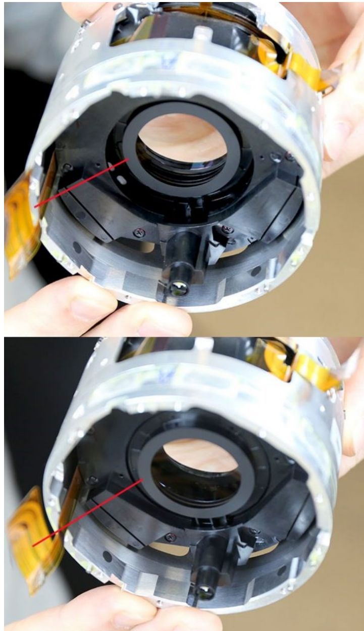
Figure 40. Autofocus lens group actuated by linear motor in its extreme positions on a Sony 70-200 mm F/2.8 GM lens. [59]
