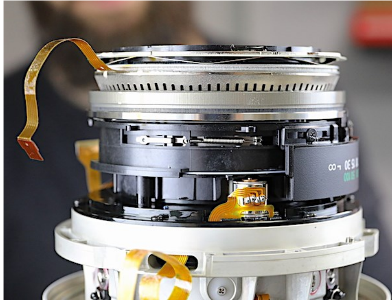
Figure 39. Canon 400mm f/2.8L IS III disassembled. The ultrasonic autofocus motor with its loading spring is the topmost part of the parts shown. [58]
