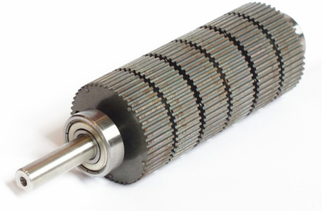
Figure 25. Stacked rotor structure of a stepper motor. This exact rotor is from a multi-stack hybrid stepper motor but the (toothed) reluctance part of the rotor is based on the same principle as variable reluctance stepper motor. [13]
