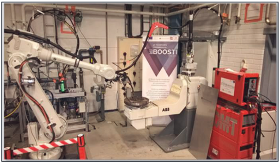
Figure 2: Wire arc additive manufacturing (WAAM) setup used in this research
