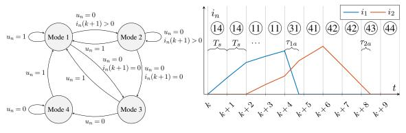
Fig. 3: State machine of branch n [7].
