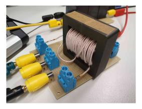
Fig. 9: Coupled inductors prototype.
