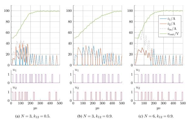
Fig. 14: Start-up behavior of the interleaved dc-dc boost converter for different N and  $k_{12}$ .
