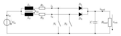
Fig. 1: Interleaved dc-dc boost converter with coupled inductors.
