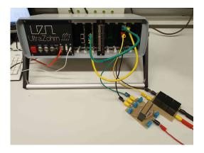
Fig. 8: Experimental setup with UltraZohm.
