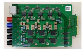
Fig. 11: GaN adapter card bottom side.
