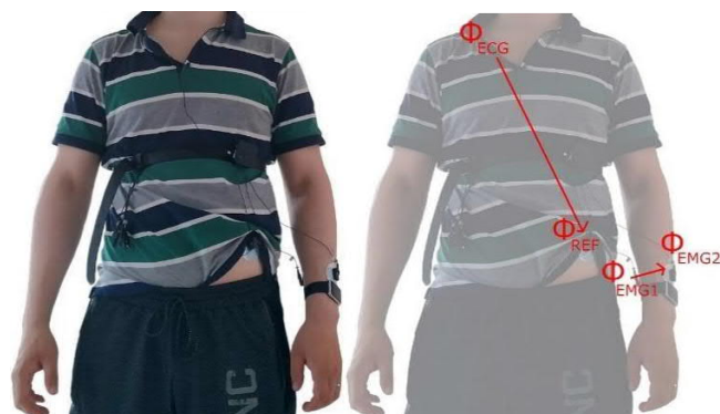
Fig. 1. Measurement setup illustrating the placement of the electrodes and wristwatch.
