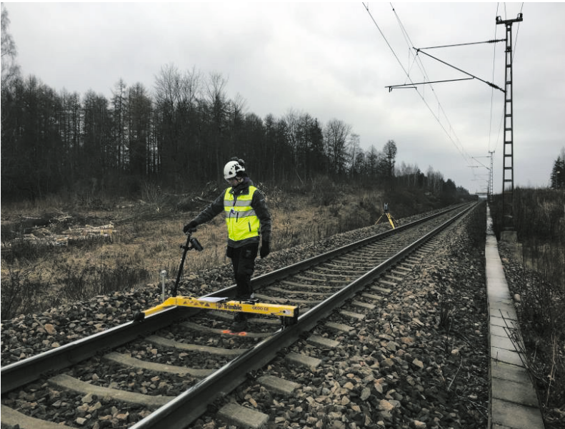
Figure 5. Lightweight track geometry measurement trolley and total station. Photo credit: Marko Happonen and Mikko Saari.
