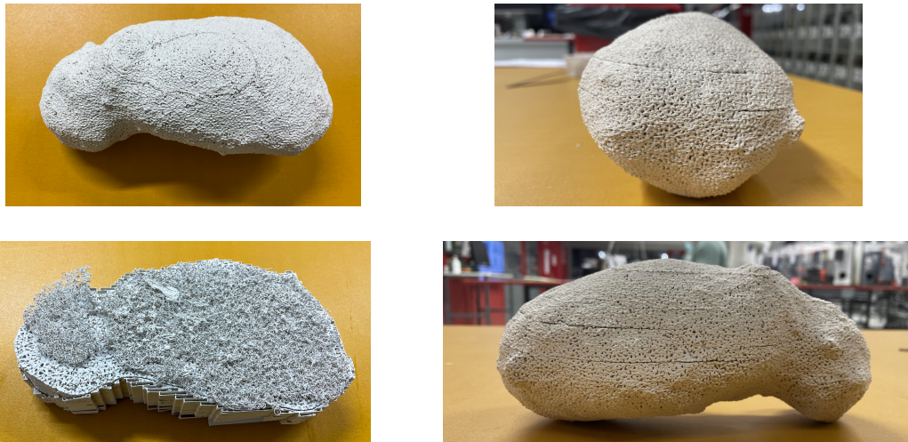
Figure 6.7 This figure shows images of the failed printing process of the Itokawa model which have defects such as cracks and layer incoherence caused by layer shifts and high temperatures and warping. The ABS650 filament was used in printing this model.
