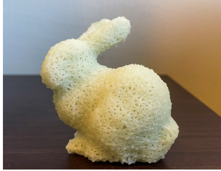
Figure 3.6 Sample 3D model of the Stanford Bunny, printed at the initial stage to test the functionality of wireframe function at Fablab.
