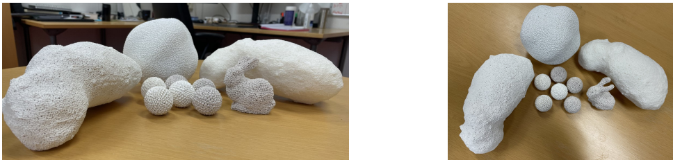
Figure 6.6 This figure shows all the bunny, spheres (3 printed with ABS450, 3 printed with ABS650), KY and Itokawa (2 printed PLA and ABS450) models together that were successfully printed at Fablab Tampere.
