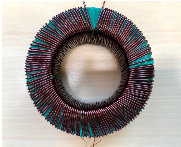
Figure 42: Completed inductor with core and windings
