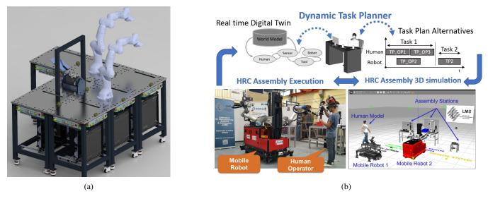
Fig. 2: (a) A reconfigurable robot workcell built from standard modules connected with plug-and-produce connectors [15]. (b) Dynamic task planning and work reorganization framework [30]–[32].
