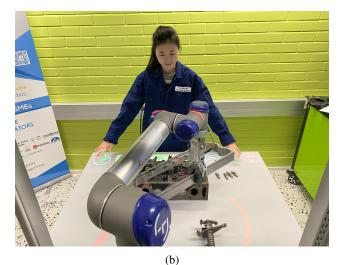
Fig. 3: (a) Flexible assembly work cell utilizing a user-friendly robot programming framework for quick programming of robots [21]. (b) Collaborative assembly with vision-based safety system [16], [36].
