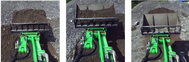
Fig. 6: Manually defined performance classes from left to right: full, half-full and empty (failed) bucket fill.
