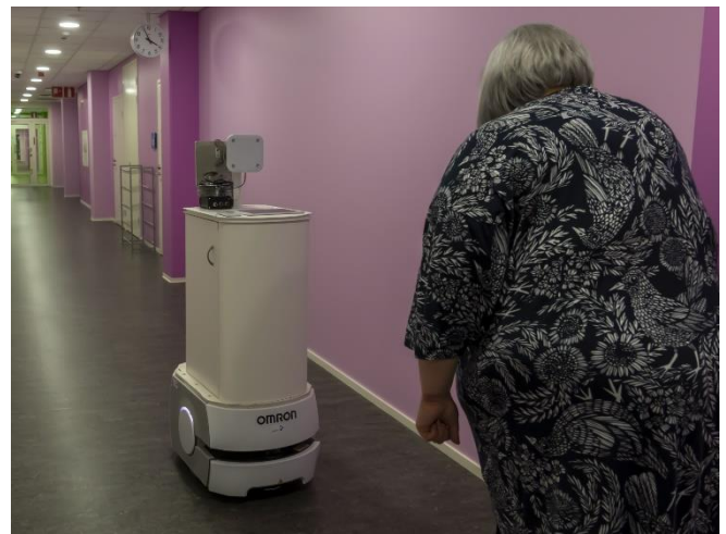
Fig. 1. A mobile robot with an integrated RFID system detects a person in the hallway and identifies her.
