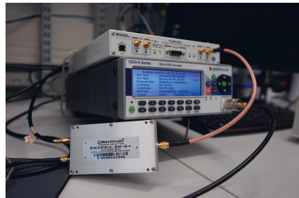
(f) Set-up for receiving GNSS+spoofer signals
