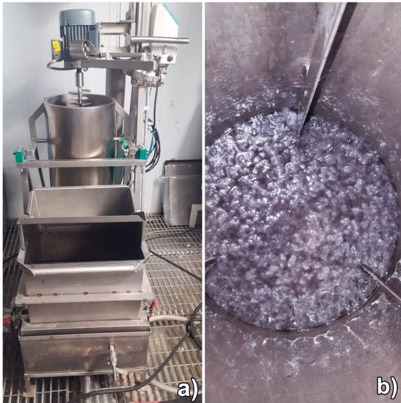
Figure 11. Laboratory scale foam forming equipment; (b) nanofibrillated cellulose-carbon nanotubes (NFC-CNT) dispersion, pulp, and water mixture before foaming in Publication IV.
