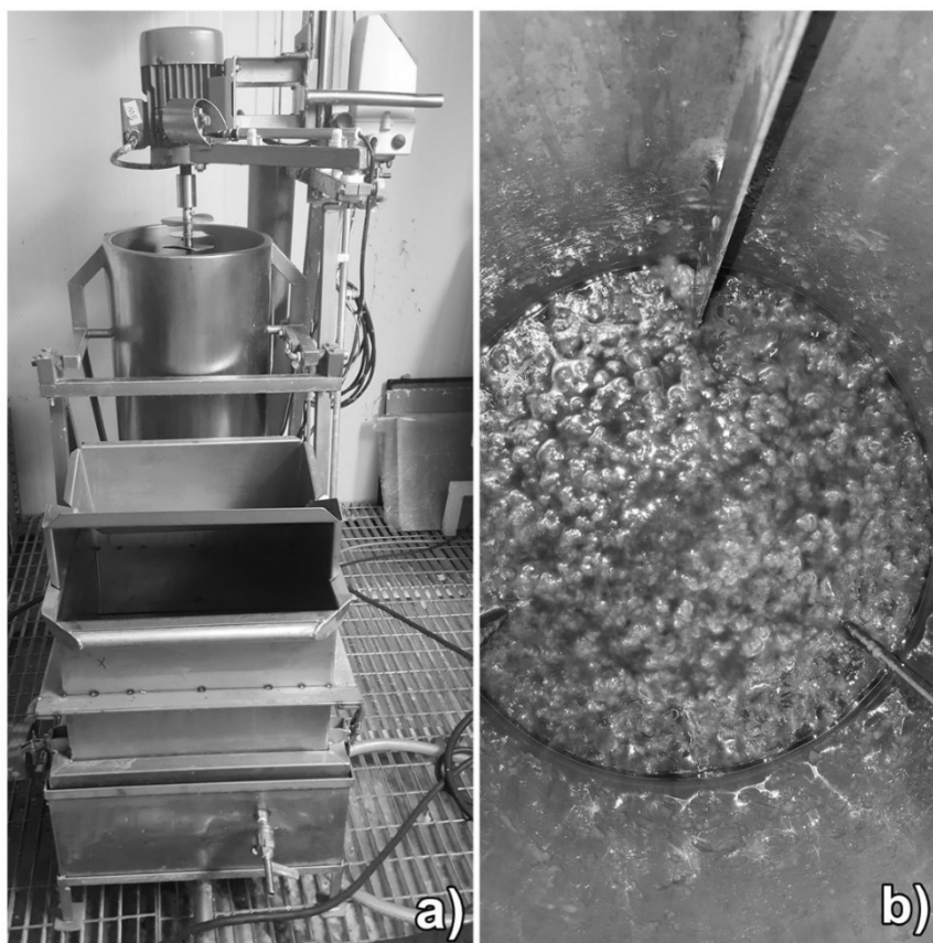
Figure 1. (a) Laboratory scale foam forming equipment; (b) nanocellulose-carbon nanotubes (NC-CNT) dispersion, pulp, and water mixture before foaming.
