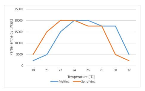
**Figure 5.** Melting and solidifying curves of the PCM product S21.
