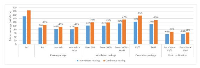
**Figure 10.** Intermittent heating vs. continuous heating: simulated relative primary energy reductions after renovating the Spanish demo building.
