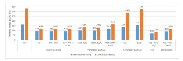
**Figure 8.** Intermittent heating vs. continuous heating: simulated relative primary energy reductions after renovating the Portuguese demo building.
