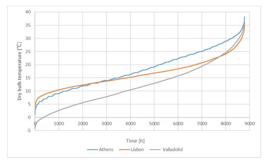
Figure 3. The duration curve of yearly outdoor temperatures in Athens, Lisbon and Valladolid.
