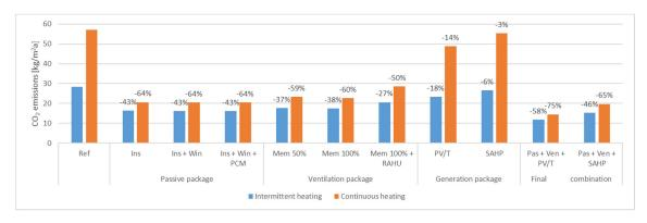
**Figure 9.** Intermittent heating vs. continuous heating: simulated relative CO<sub>2</sub> emissions reductions after renovating the Portuguese demo building.
