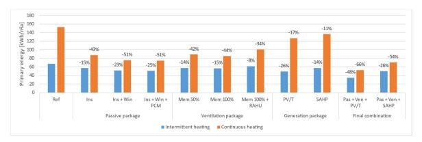
**Figure 6.** Intermittent heating vs. continuous heating: simulated relative primary energy reductions after renovating the Greek demo building.
