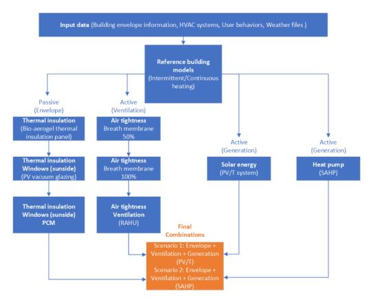
Figure 4. Simulation of retrofit packages in IDA ICE.
