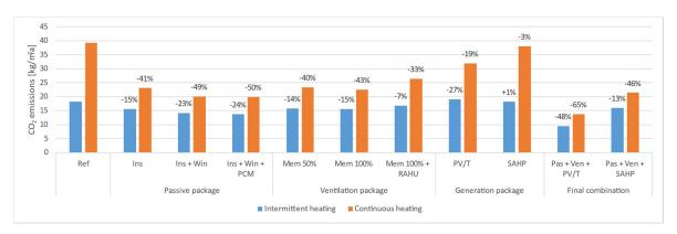
**Figure 7.** Intermittent heating vs. continuous heating: simulated relative CO<sub>2</sub> emissions reductions after renovating the Greek demo building.
