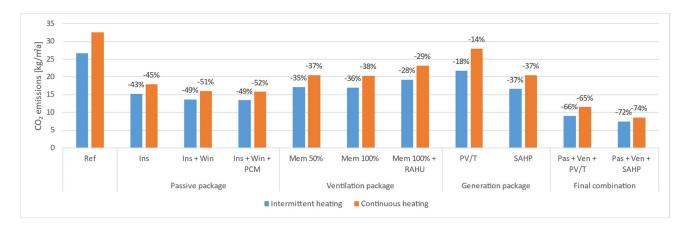
**Figure 11.** Intermittent heating vs. continuous heating: simulated relative CO<sub>2</sub> emissions reductions after renovating the Spanish demo building.
