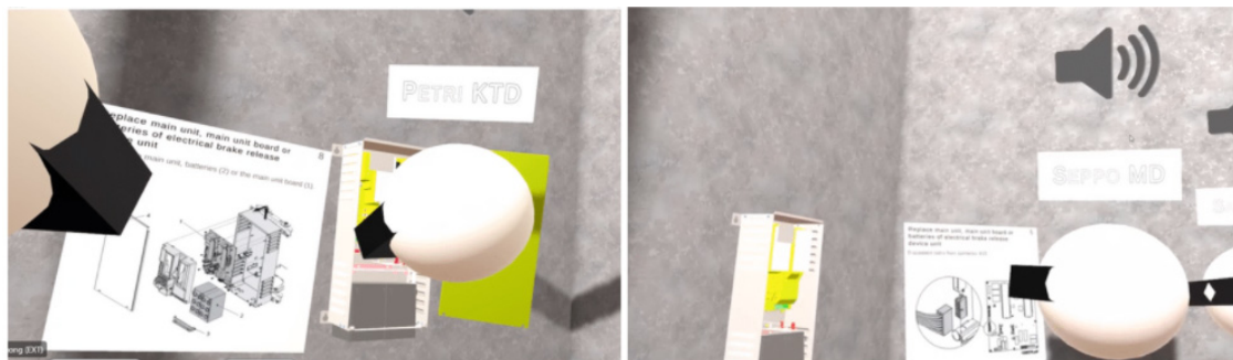
Figure 2. Screenshot of collaborative review of technical documentation in VR. A user is immersed in VR and looking at the avatars of two other users, complete with name labels for identification.
