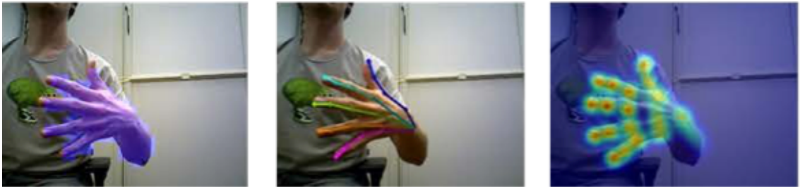
Figure 4.2 The images of hand mask (left), the detected 2D hand pose (middle) and the joint heatmaps (right) in OneHand10K (Zimmermann and Brox 2017)
