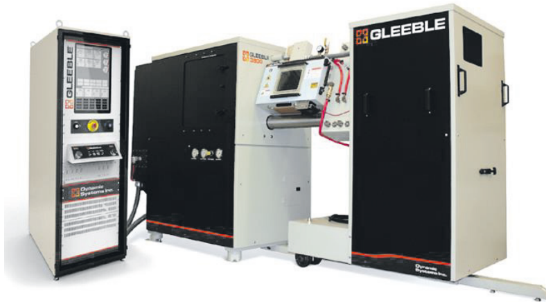
Figure 2. Gleeble 3800 thermomechanical physical simulation system. Courtesy of Dynamic Systems Inc. [149]
