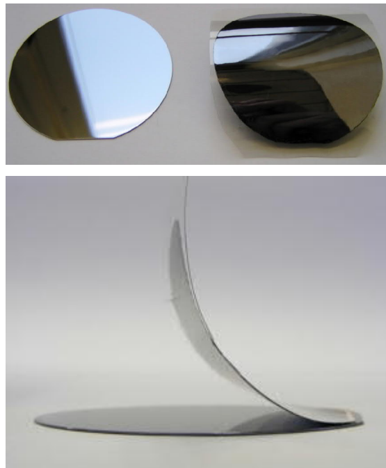
Fig. 4 Wafer-sized thin-film structures retrieved from 2-in (upper) and 4-in (lower) diameter GaAs substrates by epitaxial lift-off using a flexible carrier/handle.
