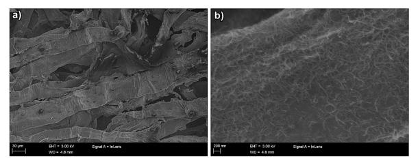
**Figure 2.** (a) Homogenous CNT coverage over cellulose fibers and (b) carbon nanotube percolation network on the surface of cellulose fiber.
