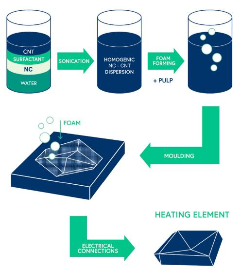
Figure 3. Manufacturing process of heating element prototype Salmiakki.
