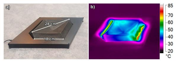
**Figure 4.** (a) Visual image of plywood mounted Salmiakki with dimensions and (b) Infrared camera image of heating element prototype Salmiakki at steady state in room temperature.
