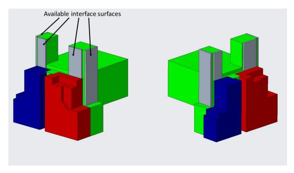
Figure 13. Available space with available sling interface surfaces
