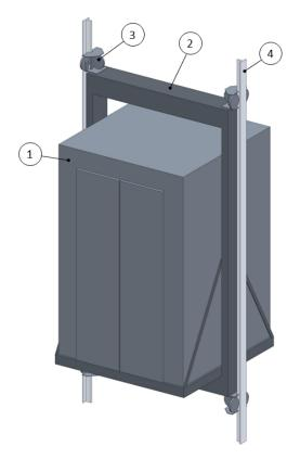
**Figure 1.** A visualization of the main components of elevator guiding system with a car enclosure. Components as numbered: 1 – car enclosure, 2 – sling, 3 – guide shoe, 4 – guide rail
