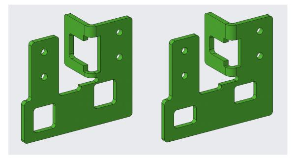
*Figure 18.* Example of how reducing the height of dampers enables higher strength of structures. Original is on the left and on the right is the reduced height version
