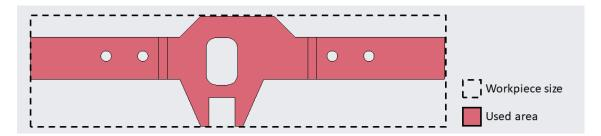
Figure 16. Safety throat integrating frame part with required workpiece size
