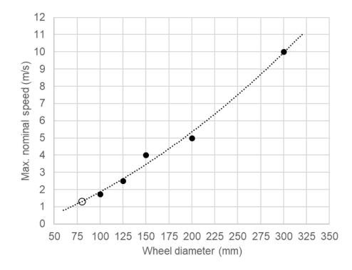
*Figure 5.* Extrapolated plot of maximum nominal speed in relation to wheel diameter on elevator car side
