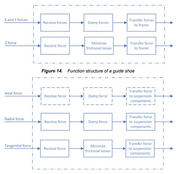
*Figure 15.* Function structure of a guide shoe contacting element
