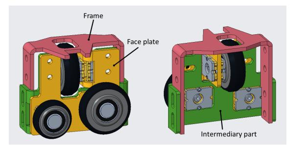
*Figure 19.* Variant E3\_1 body parts named
