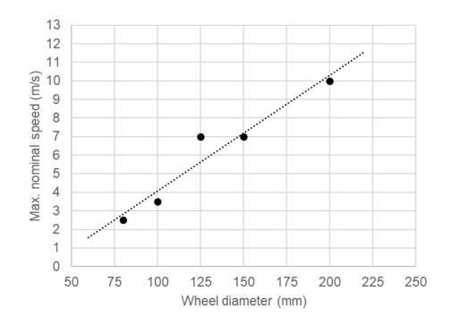
*Figure 6.* Extrapolated plot of maximum nominal speed in relation to wheel diameter on counterweight side
