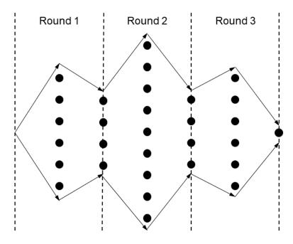
Figure 23. Divergence and convergence through embodiment design phase
