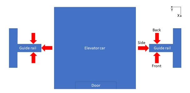
Figure 4. Directions of restriction. NOTE: not in scale
