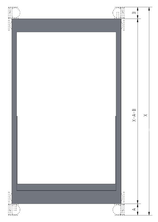
Figure 3. Possible height reduction enabled by sling integrated guide shoes
