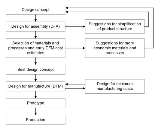
Figure 11. A typical process of utilizing DFMA according to [28]
