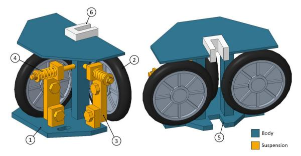
**Figure 2.** Model of a traditional type of spring suspended roller guide. Components as numbered: 1 – body, 2 – roller, 3 – lever arm, 4 – spring system, 5 – safety throat, 6 – removable slider
