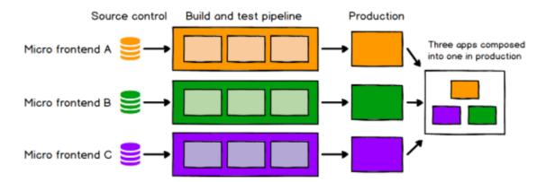
Figure 2.3 Each micro frontend is deployed to production independently [6]
