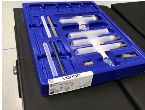
Figure 3. Shielded applicator set used in dose measurements. This applicator set included five applicators with different diameters, as well as quarter cylinders to be placed inside the applicator to implement shielding. The applicators were approximately 15 cm in length.
