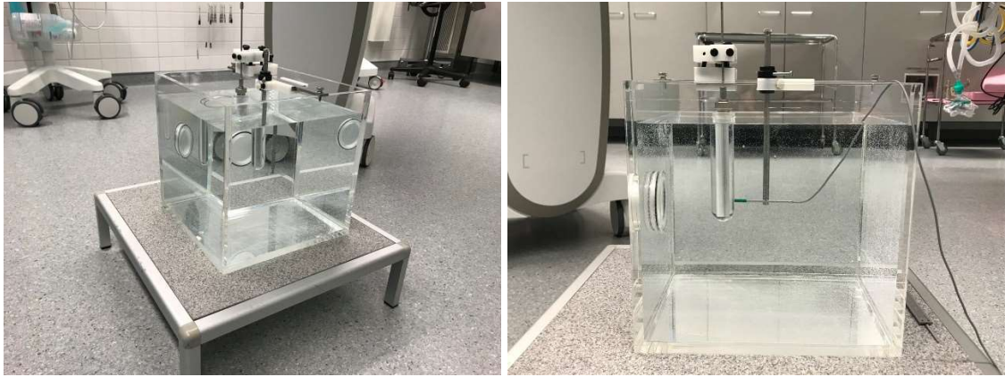
Figure 4. Pictured in this figure is the experiment setup. The applicator was submerged into a 30 cm × 30 cm × 30 cm container filled with tap water, and the detector was placed on its side with the shielding rotated appropriately for each measurement.
