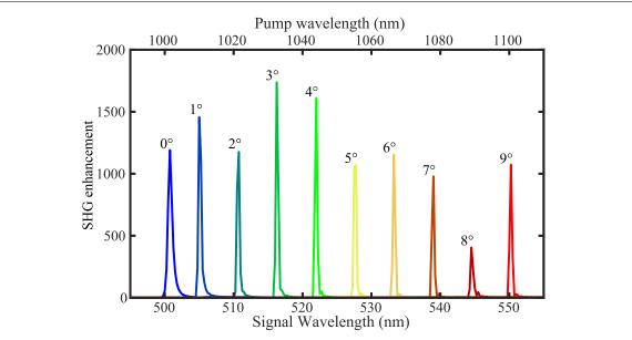
**Figure 4.** Tunable frequency conversion of narrowband laser pulses ( $\Delta \lambda_{\rm L} \approx 1$  nm) via angle-dependent SHG. The SHG signals are normalized to the non-resonant case (5 nm off the SLR wavelength).
