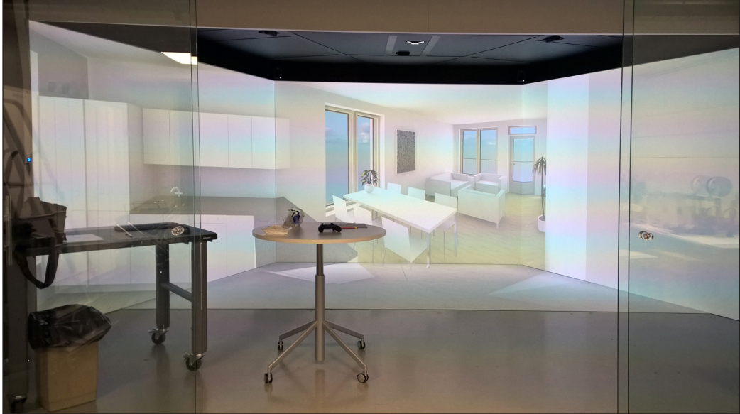
Figure 3: 3D CAVE virtual environment with a test flat projected onto the walls and floor.
