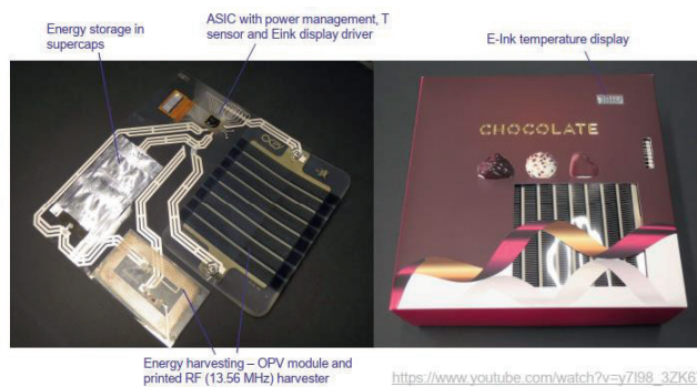
Figure 4. Pictures of energy autonomous temperature sensor mounted inside a smart chocolate box [73].
