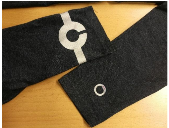
Fig. 9. Practical integration into clothing: Electro-textile wrist antenna and ID ring ironed directly into a shirt.
