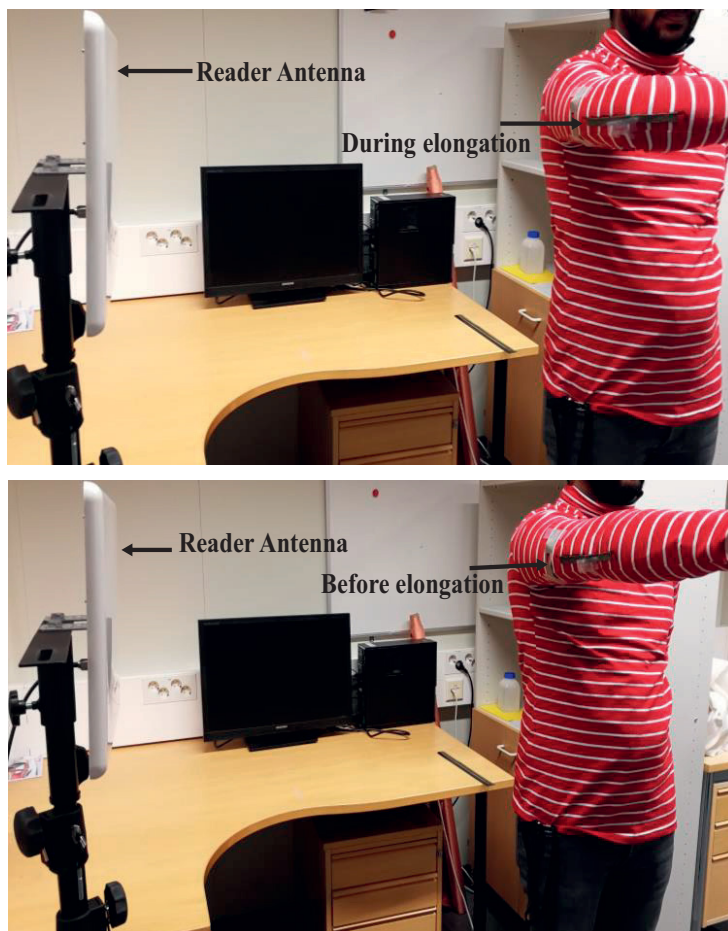
Figure 28. The measurement setup of a body movement-based sensor in an office environment, bent (top), and straight elbow (bottom) [Publication II].
