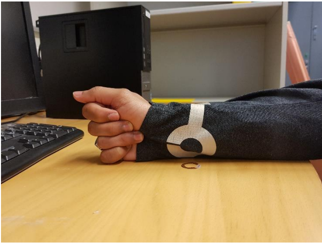
Fig. 10. Shirt-integrated wrist antenna is used to activate an ID ring on a table. This setup showed a read range of 93 cm.
