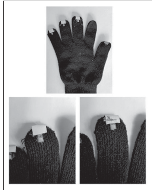
Figure 6. Interface glove from non-stretchable electro-textile: palm side of the glove (top), glued integrated circuit (IC) attachment (bottom left), and embroidered IC attachment (bottom right).
