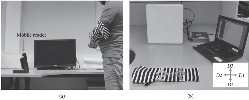
FIGURE 3: (a) Platform testing with a mobile reader and (b) M6 reader.
