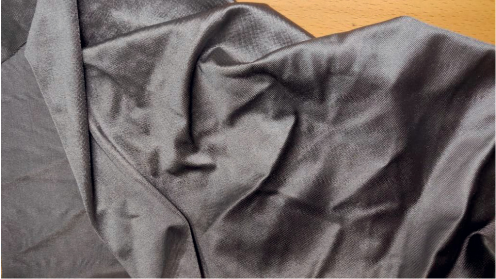
Figure 9. Less EMF stretch conductive fabric.
