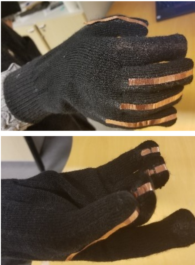
Fig. 3. Off-status (top) and on-status (bottom) of the glove-integrated user interface.
