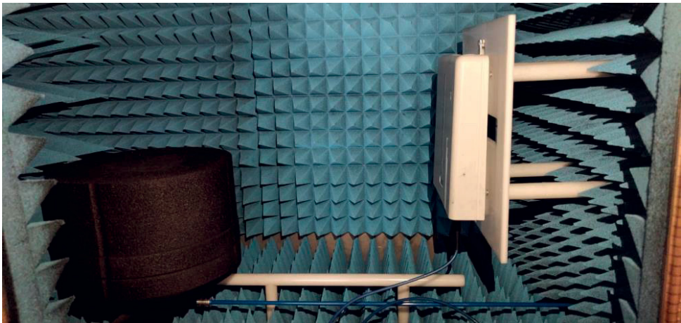
Figure 18. Anechoic chamber for Voyantic Tagformance measurement system used for initial wireless evaluation of prototypes in this thesis.
