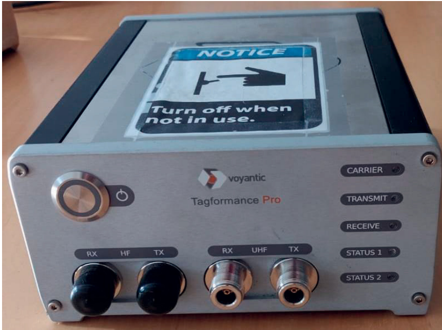
Figure 19. Voyantic Tagformance measurement system used for initial wireless evaluation of prototypes in this thesis.
