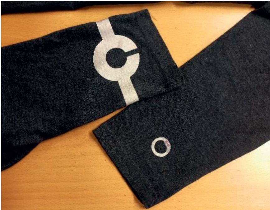
Figure 23. First body movement–based interaction solution, a wrist antenna and small ID ring integrated into the shirtsleeve [Publication I].
