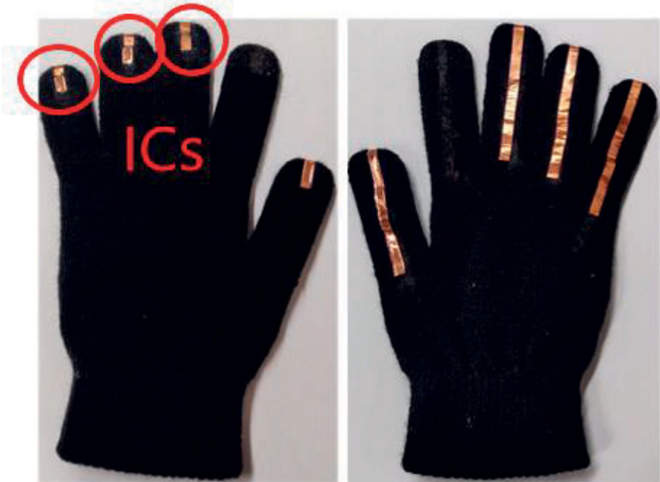
Figure 40. AAC gloves tested in a home environment (left) and an office environment (right) with mobile and M6 RFID readers [Publication VIII].
