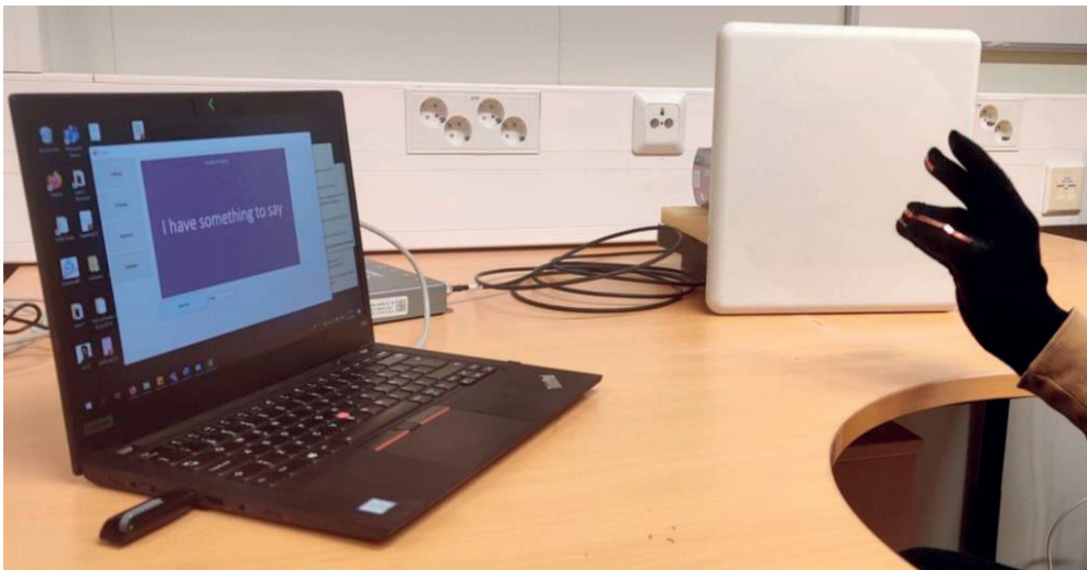
Figure 42. Testing environment of AAC gloves with an M6 RFID reader in an office environment [Publication VIII].
