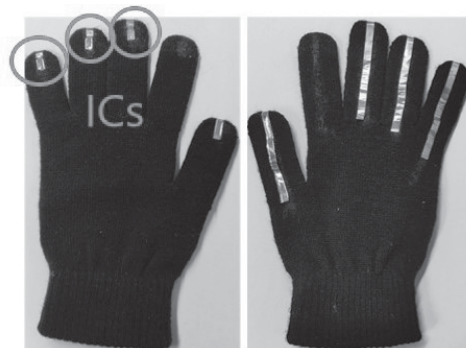
Fig. 1. Integrated copper tape antennas on the palm side of an intelligent glove (left) and on the backside of an intelligent glove (right).
