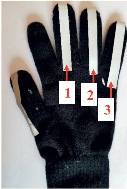
Figure 38. The glove platform fabricated from non-stretchable conductive textile material [Publication VII].
