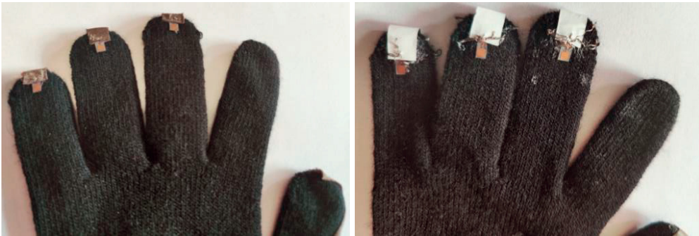
Figure 7. Embroidered interconnections of IC and antennas.
