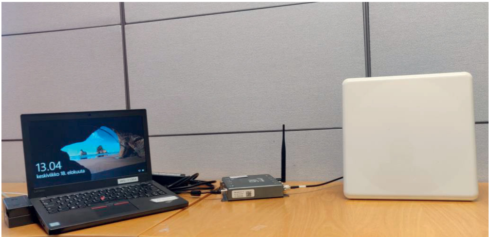
Figure 20. Mercury ThingMagic M6 RFID reader system used for practical testing in this thesis.
