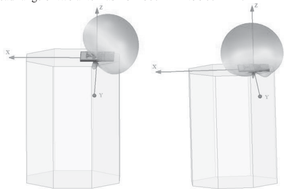
Fig. 4. Simulated 3D gain pattern of the Quasi-Yagi antenna (left side) and dipole based reflector (right side) at 915 MHz.
